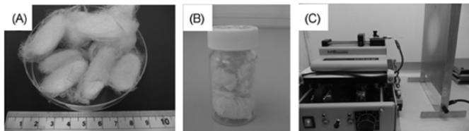
Figure 7. This image shows the transformation of silk fibroin from (A) unprocessed B. mori silkworm cocoon to (B) extracted, lyophilized silk fibroin and (C) final, electrospun silk fibroin mat [80].
