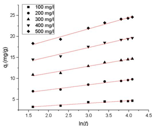
**Figure 3.** *Elovich* model for acid dye adsorption on wool fiber pre-treated with *n*-pentanol at different initial dye concentrations
