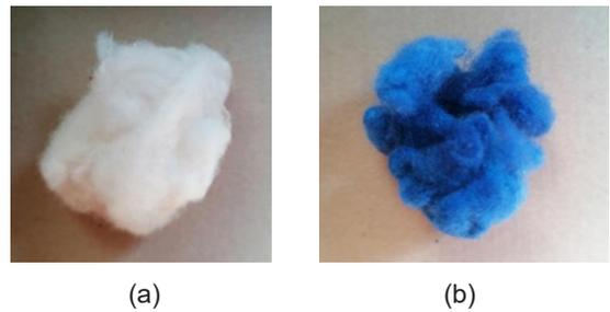
**Figure 2.** The appearance of the wool fiber after pre-treatment with alcohol (a) and after the dyeing of pre-treated wool fiber (b)
