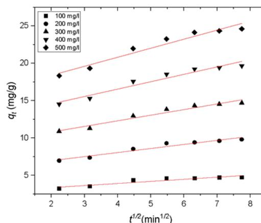
**Figure 4.** *Weber-Morris* kinetic model for acid dye adsorption onto wool fiber pre-treated with *n*-pentanol
