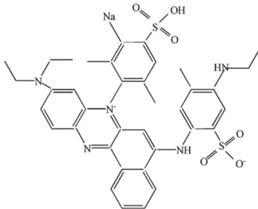
**Figure 1.** The chemical structure of Supramin Blau acid dye
