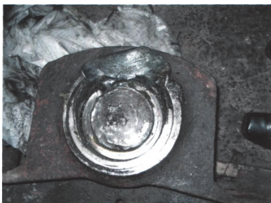
Figure 7: Aspect of the deformed area of the grease box
