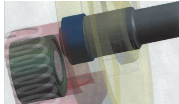
Figure 6: Detaching the grease box from the end of the axle
