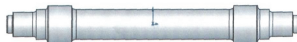
Figure 14: Drawing of the OR 1-1 axis obtained by cutting the ends of an OR 1 axis
