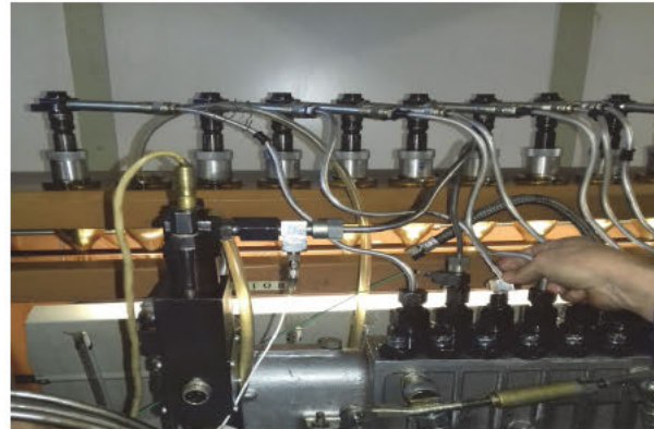
Figure 3: High pressure pipes with original engine and a special assembly (indicated by an arrow) for measuring the stroke of the injector needle
