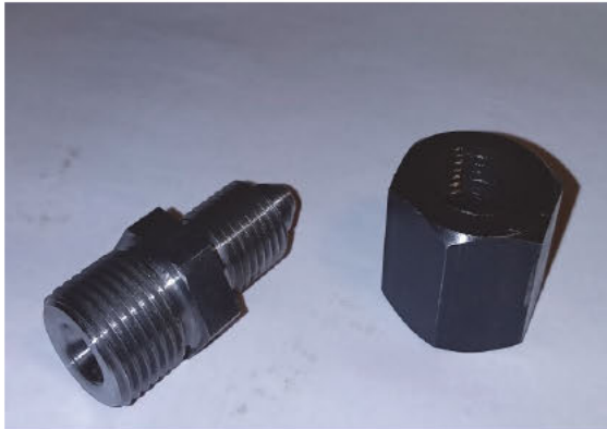
Figure 2: Specially designed adapters and nuts that have injectors a right-hand thread on one end and a left-hand thread on the other end
