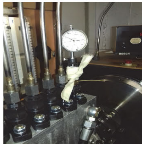
Figure 5: Measuring assembly for determining the pre-lift of the element for P500 family pumps
