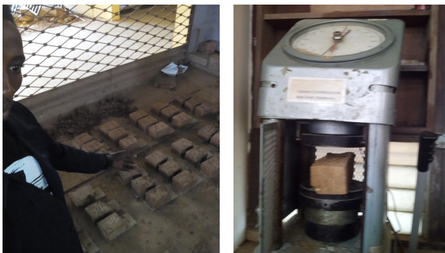
Figure 3: Compressive testing machine
