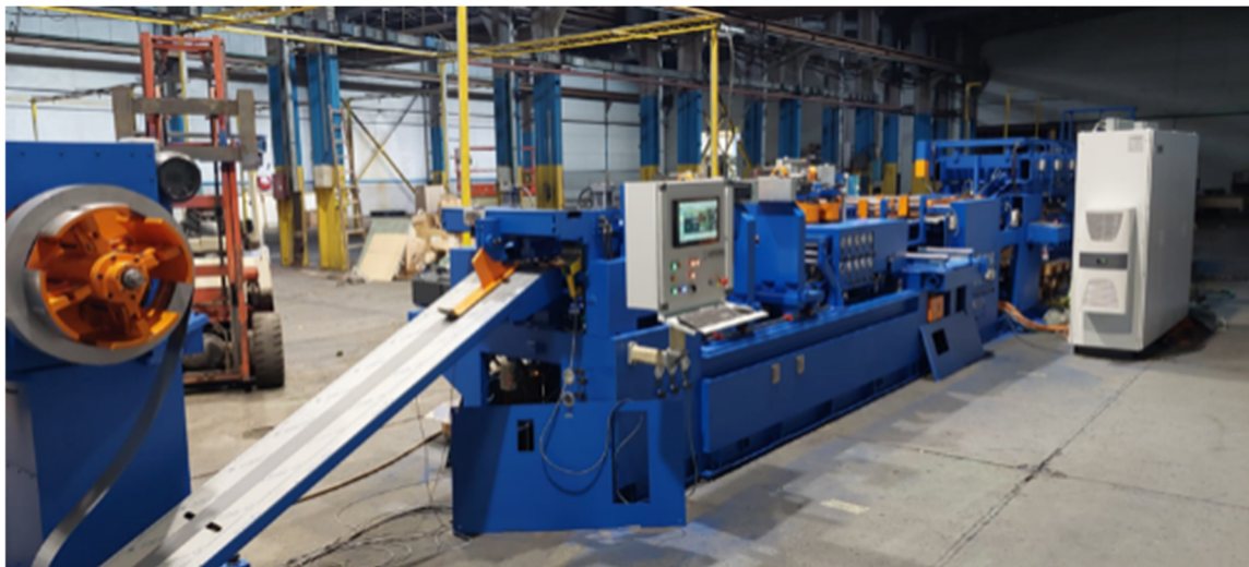
Figure 1: Automated transformer magnetic core cutting line
