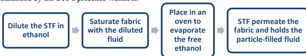
Figure 8: Process of STF incorporation to fabric
