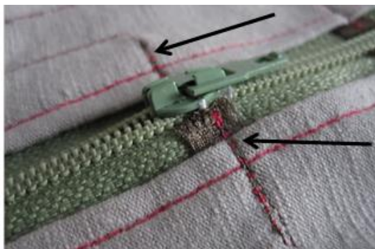
Figure 7: Switching via zip via conductive threads (arrows) [20,21]
