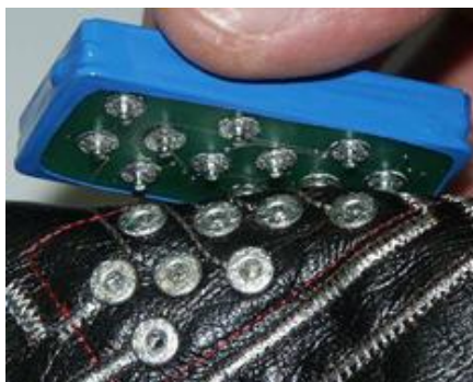
Figure 2: Putting the module on the prepared piece of clothing using snap on button [5]
