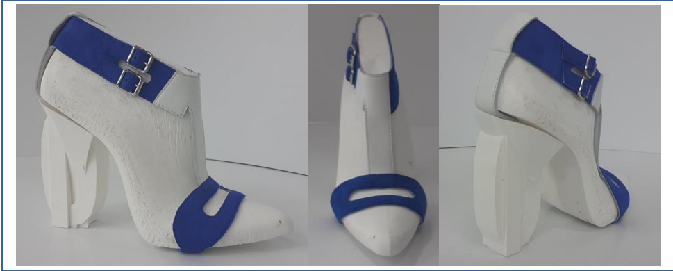
Figure 6: Different views of sandal model 1 during production process over 3D printed last.
