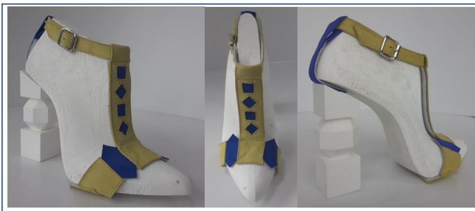
Figure 8: Different views of sandal model 3during production process over 3D printed last.
