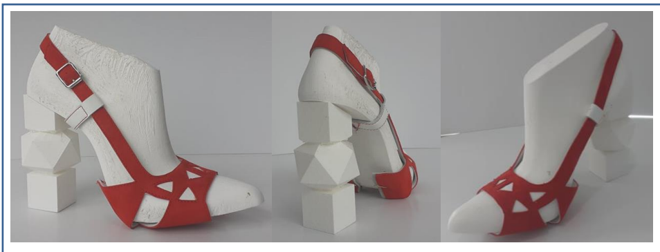
Figure 7: Different views of sandal model 2 during production process over 3D printed last.
