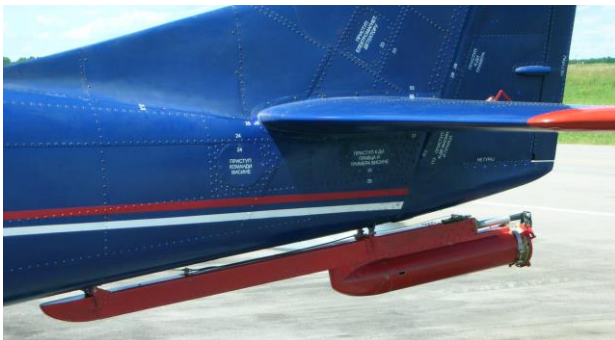
Figure 2. Antispin parachute system on airplane Lasta 95
