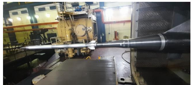
Figure 2. Supersonic projectile model in the VTI T-38 test section
