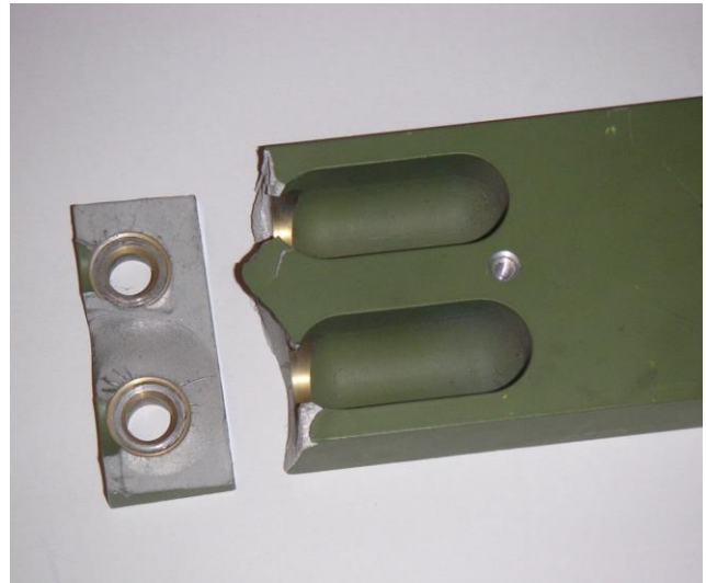
Fig. 5 The fracture appearance of the wing-fuselage connection part after the fatigue test
