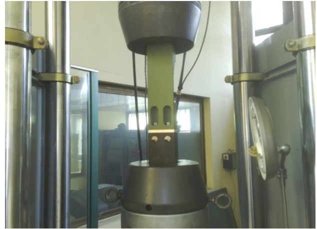
Fig. 4 Part of the wing fuselage connection
