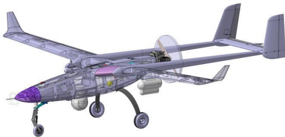
Figure 4. OUT unit attached to the wing pylon
