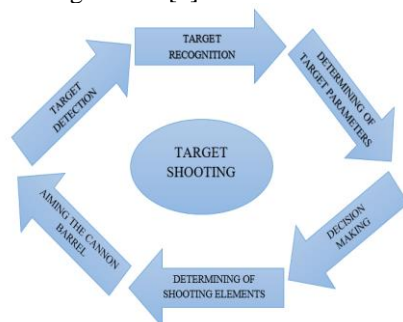
Figure 1. Fire control system procedure
