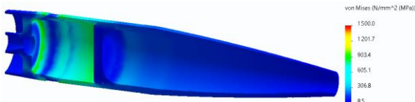
Figure 7. Stress condition for a model with 9 kg propellant charge
