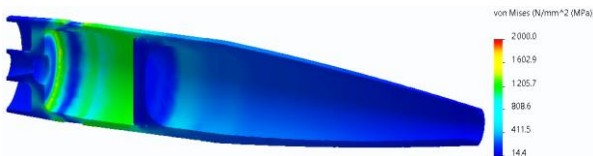
Figure 8. Stress condition for a model with 13 kg propellant charge
