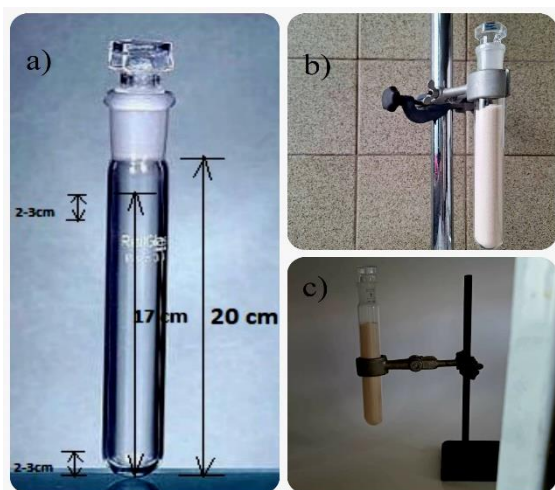
Figure 3. a) Test tube for samples with its dimensions, b) sample exposed to light and ambient temperature, c) sample stored in a dark on ambient temperature
