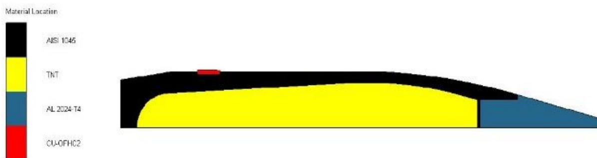
Figure 1. Artillery projectile 105mm M1, 3D quarter numerical model with material assignment
