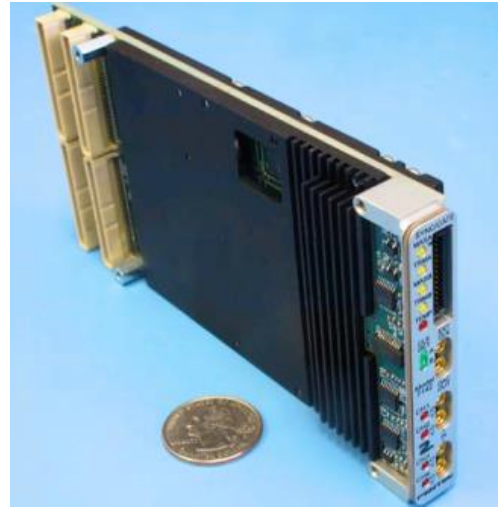
Picture 3: The Pentek 7142 FPGA transceiver.
