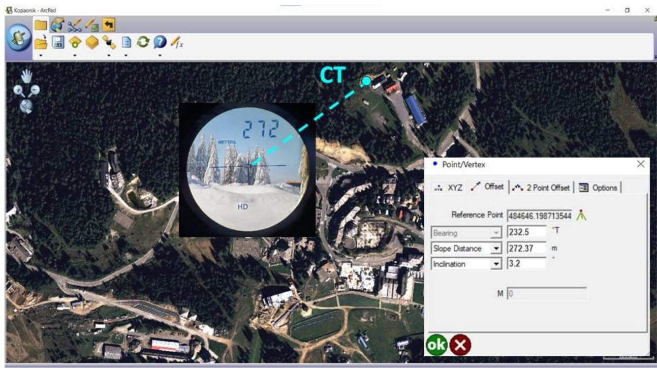
Figure 7. Locating a distant target by integrating mobile devices
