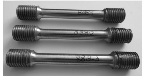
Figure 4. Geometry of specimens prepared for tensile tests [1]
