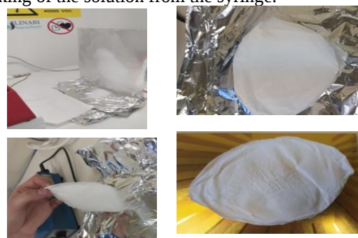
Figure 1. Nanofiber membranes obtained by electrospinning.
