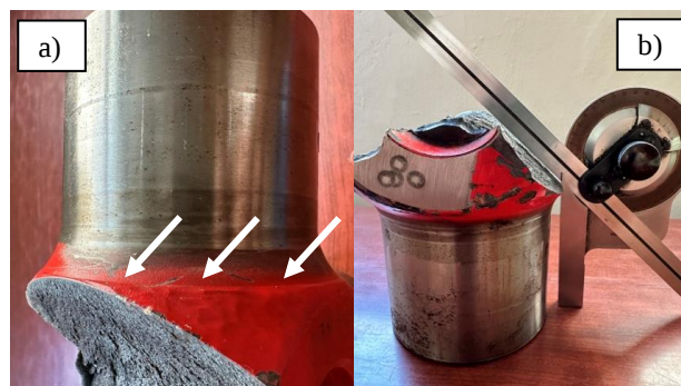
Figure 2.2. Fracture of the sleeve of the UCJ
