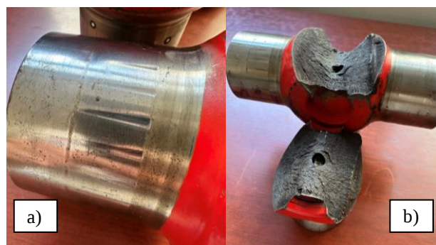
Figure 2.1. a) Surface damage of the sleeve in the form of local plastic deformations, b) volumetric damage of the sleeve in the form of breakage
