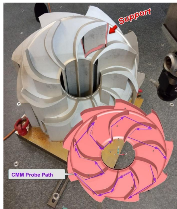
Figure 4. Diffuser N°3 on the CMM & touch trigger probe measuring path
