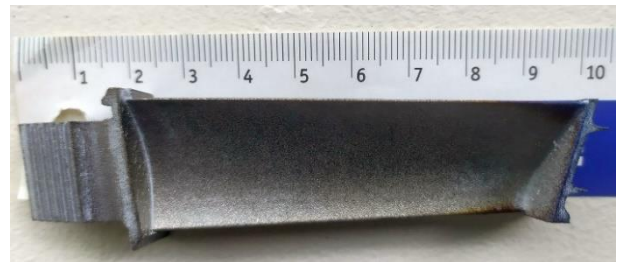
Figure 6. Turbine Blade built on an AM machine
