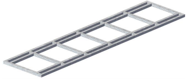
Fig.6. A finite element model of the removable module
