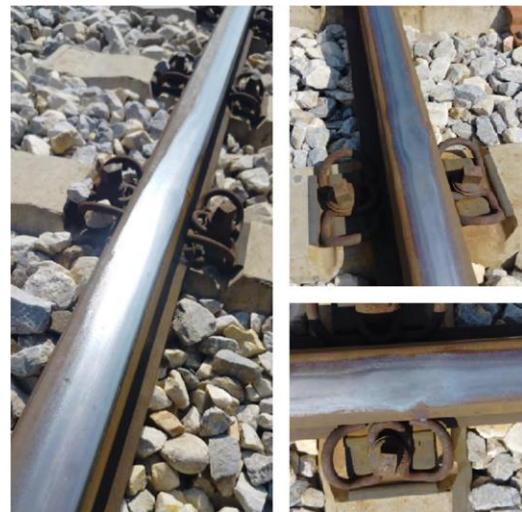
Fig. 5. Rail distortion caused by struggling train traction.
