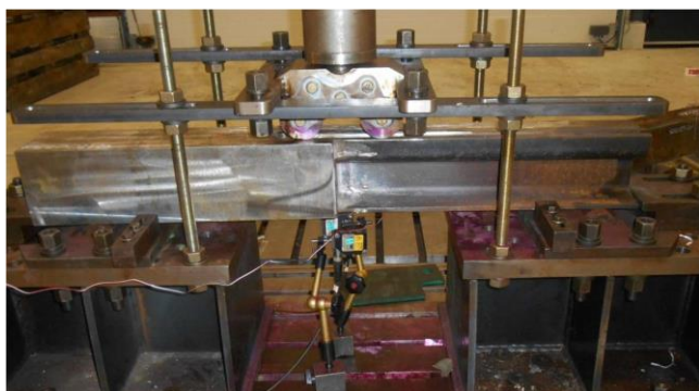
Fig. 6. Fracture testing machine
