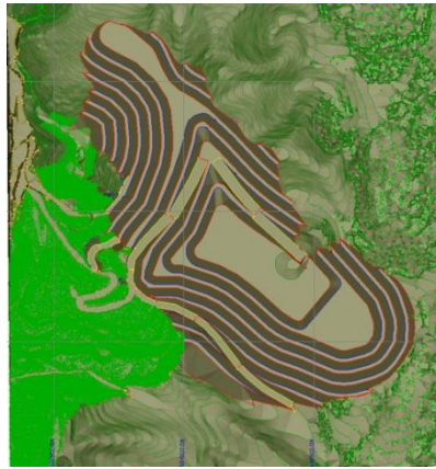
Figure 2. Designed final contour of the Saraka landfill
