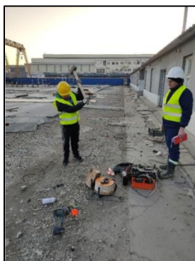
Figure 3. Presentation of seismic refraction measurements in the field
