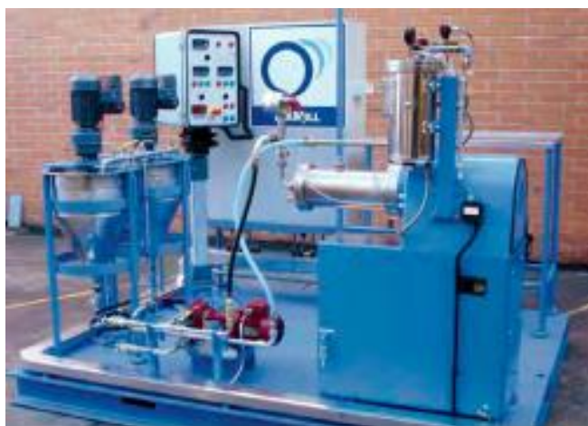
Figure 2-2. Laboratory M4 (4L) IsaMill test rig [1]
