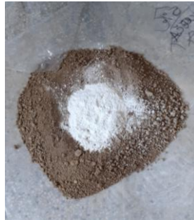
Figure 2. Homogenization material of subsoil with 5% lime
