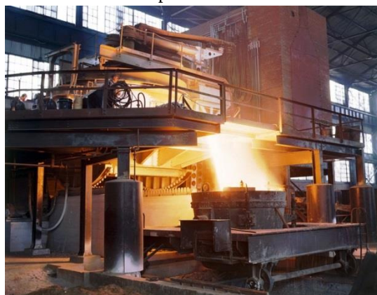
Figure 2. Steel production in an electric arc furnace (5)
