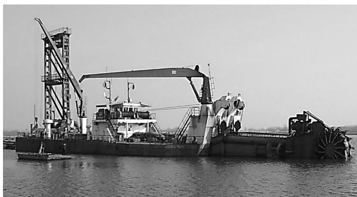
Figure 3, Floating suction dredger "Kovin I" with UCW 450 cutting wheel
