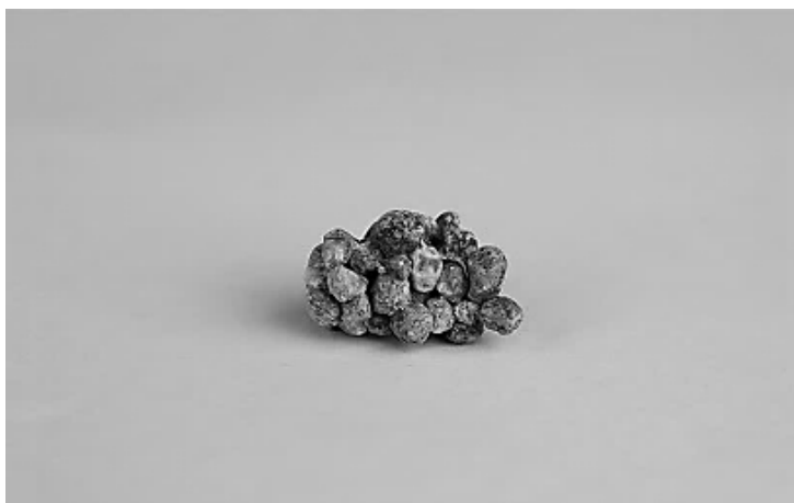
Figure 4, Limestone's tendency to clump can complicate the pelletizing process, as any imbalance may lead to the formation of clumped pellets, often referred to as "raspberries," as illustrated here
