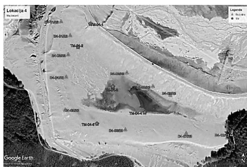
Figure 4, Schedule of exploration works - Site 4 (exploration boreholes marked B4 and geophysical tests marked TM04)
