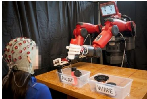
Figure 8. The feedback system enables human operators to correct the robot's choice in real-time. After (Robohub, n.d.)
