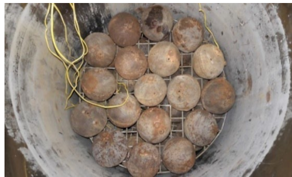
Figure 3 Arrangement of PCM capsules in the TES tank
