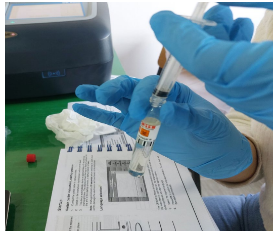
Figure 18. Putting the specific amount of sample into the LCK cuvette
