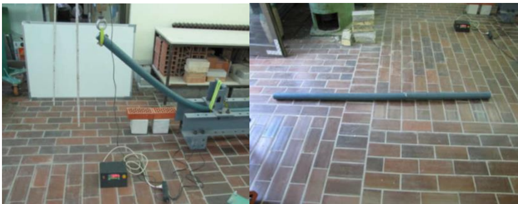
Picture 2. Bending testing of circular cross-section columns until failure and reversible deformations on the sample after testing [7]
