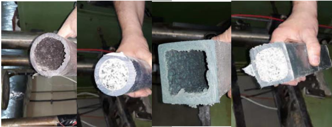
Picture 1. The column samples during testing: circular and square cross-sections (hollow and filled) [7]
