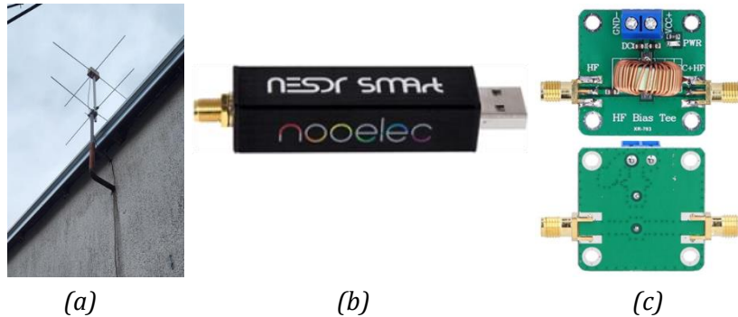
Figure 2. Equipment: (a) The KX-137 antenna system; (b) Nooelec RTL-SDR v5 device; and (c) Bias T Modul.
