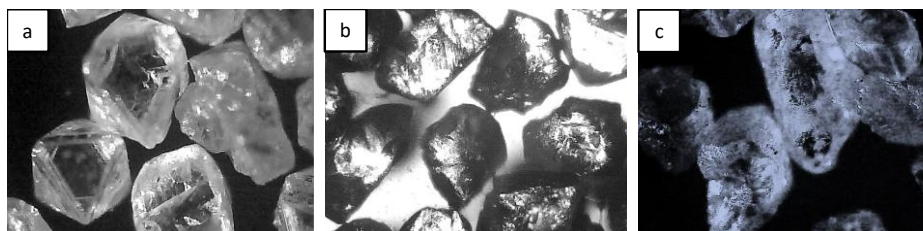
Figure 1 Images of diamond crystals at foam separation (a,b) with fixed asphaltene-resin cut fraction (c)
