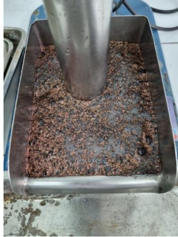
Figure 4 The image of floating copper particles in the copper flotation stage
