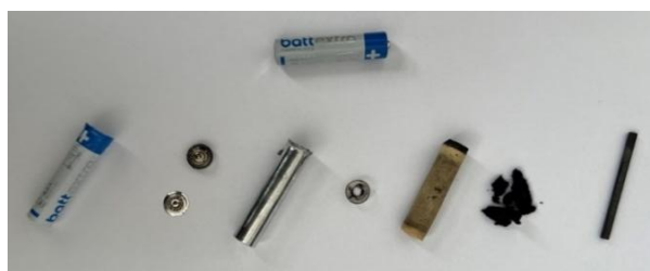
Figure 1 Zn-C batteries and their individual parts
