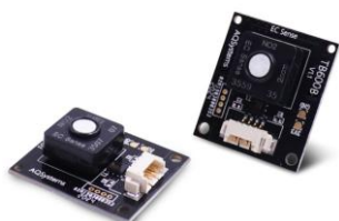
Figure 3a EC Sense NO 2 Gas Sensor Module TB600B [9]
