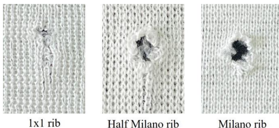
Figure 5: The surface appearance of organic wool double weft knitted fabrics in three knit structures - 1×1 rib, half Milano rib, and Milano rib, at 10 × magnifications following the evaluation of their strength properties
