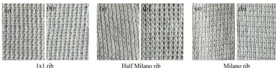
Figure 1: The surface appearance of organic wool double weft knitted fabrics in 1x1 rib, half Milano rib, and Milano rib at 10× magnification: (a) face side of fabric, (b) back side of fabric
