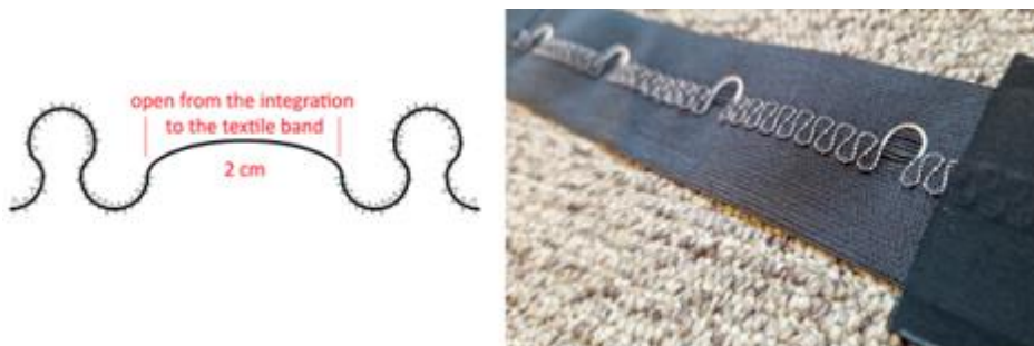
Figure 3: Interconnect ribbon with conductive yarn that was attached onto ribbon in a horse-shoe shape [16]
