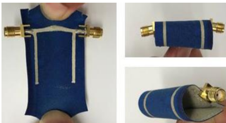
Figure 1: Stretchable and washable filter ink printed directly on stretchable textile [14]
