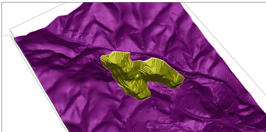
Figure 2. Whittle 3D view of the optimal pit number 36
