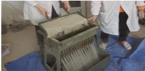
Figure 1. Shortening of the sample on the Jones riffle splitter
