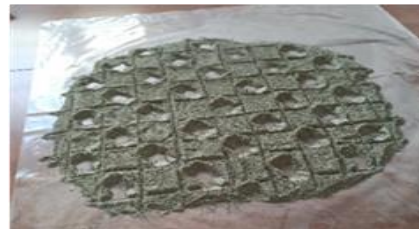
Figure 2. Taking the representative samples by chessboard method for
