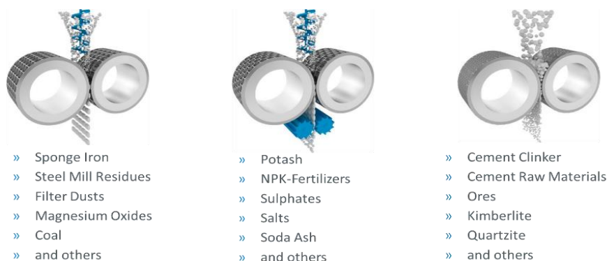
Figure1. Overview of roller pressing applications; left Briquetting, middle Compaction, right Comminution
