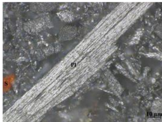
Figure 7. Irregular grain of sulfur [6]
