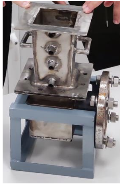
Figure 12. Assembled sintering facility
