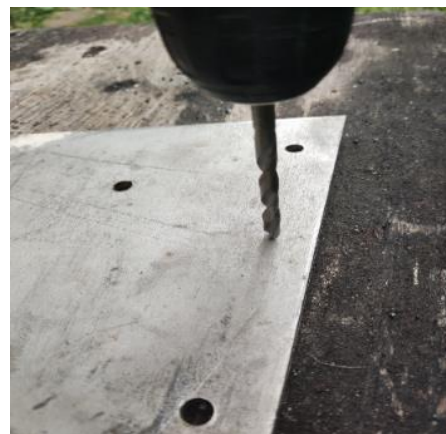
Figure 10. Forming the necessary holes for thermocouples, pressure gauge and exhaust gases
